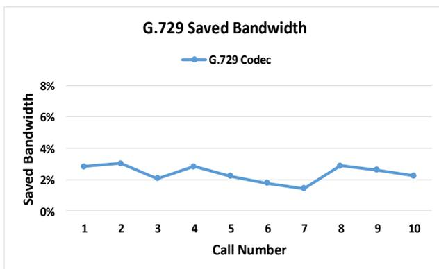
Figure 10. Saved bandwidth of the G.729 codec
