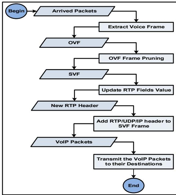
Figure 3. SS-VFP module process
