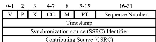
Figure 1. RTP protocol header format
