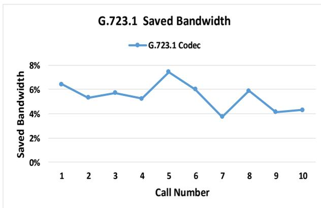
Figure 9. Saved bandwidth of the G.723.1 codec
