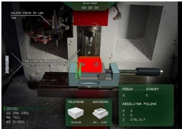
Figure 8. Output of the augmented monitoring system
