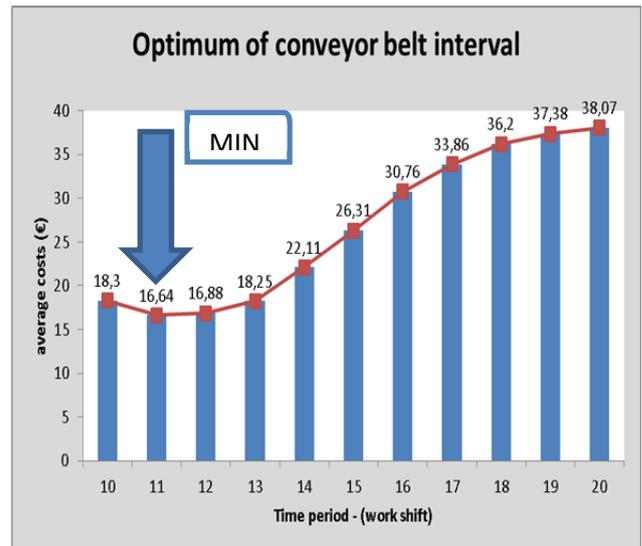
Figure 4. Optimal time interval of raw material exchange of belt conveyor
