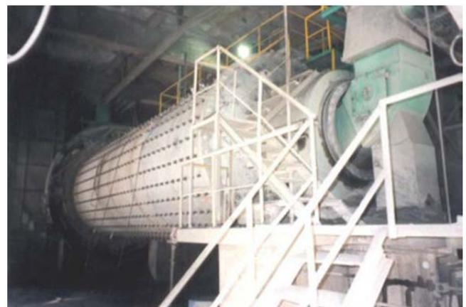
Figure 1. Ball mill in mining company
