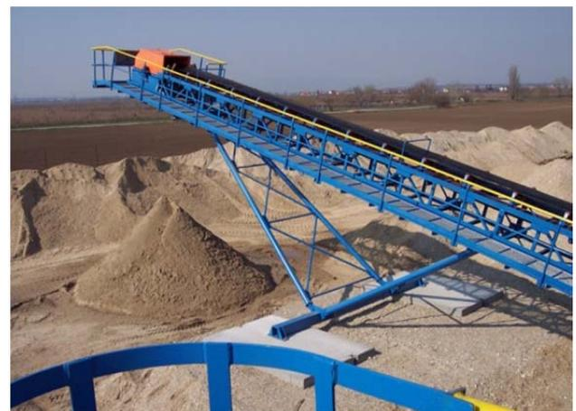
Figure 3. Belt conveyor in mining company
