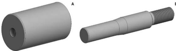
Figure 1. Cylindrical mandrels used for pulling pipes
