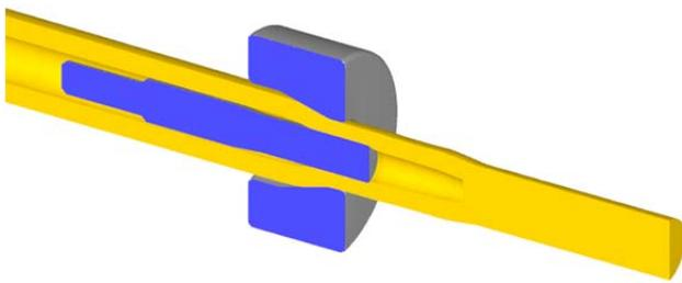
Figure 5. 3D view of the drawing process in section
