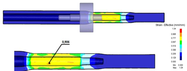
Figure 8. 3D simulation of stress effective
