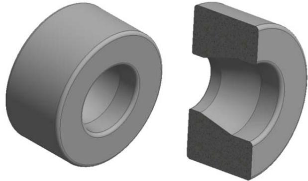
Figure 3. 3D view of the die and the die in section
