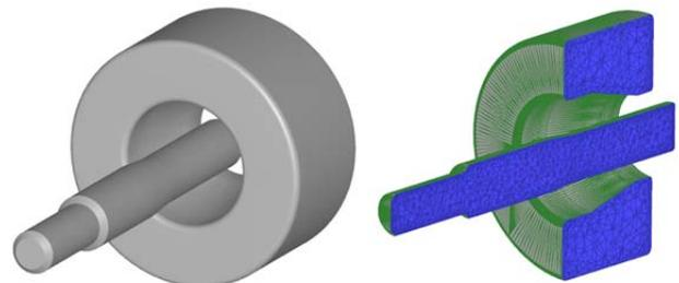
Figure 4. 3D assembly (mandrel and dies)
