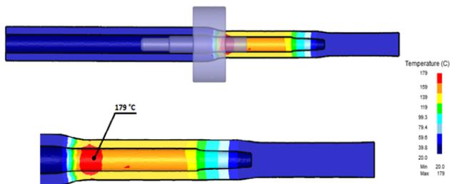
Figure 10. 3D simulation of temperature analysis of test tube
