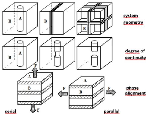
Figure 2. Characteristic parameters of composite materials [3]
