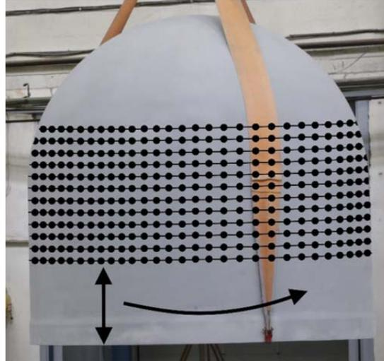
Figure 4. Example of the shape of the investigated radome with measuring points  $E_{x_i y_i}$
