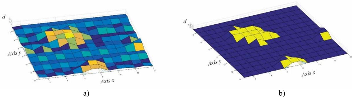
Figure 9. Graphical display of the value of  $d$  in the coordinate system  $Oxy$  (a) and the corresponding display of areas with excess level  $d_A$  (b)
