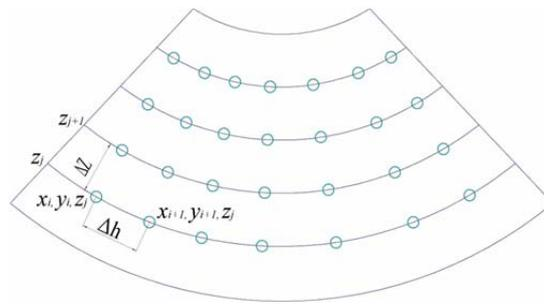
Figure 6. Layout of the points on the scan cylinder
