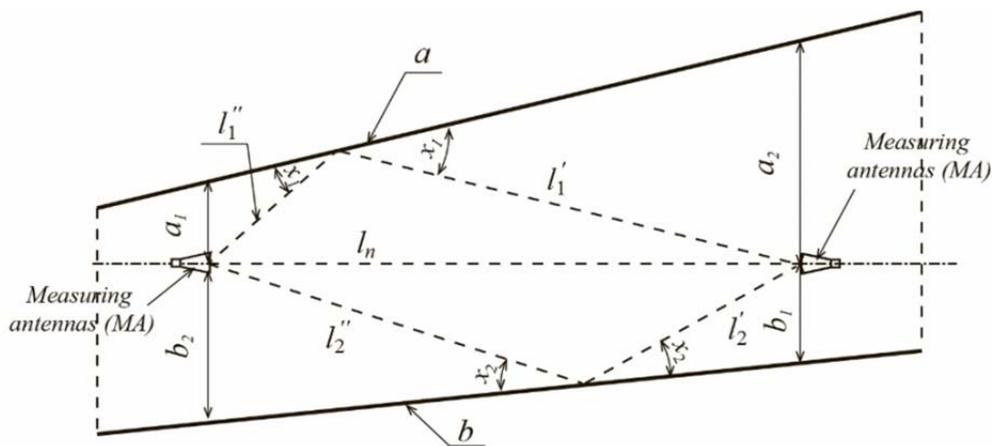
Figure 2. Measuring antennas location at the polygon. View from above
