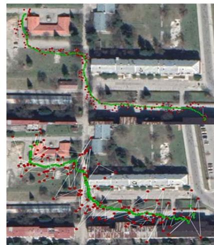
Figure 6. Comparison of the receiver position calculation (A50 on upper image, Xiaomi on lower image, with (green) and without Kalman filter(red))
