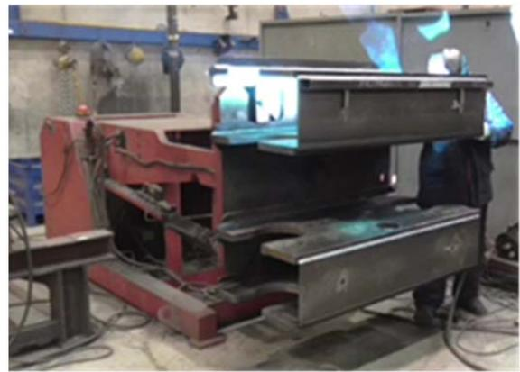
Figure 14. Original positioner for Fahrschemel welding
