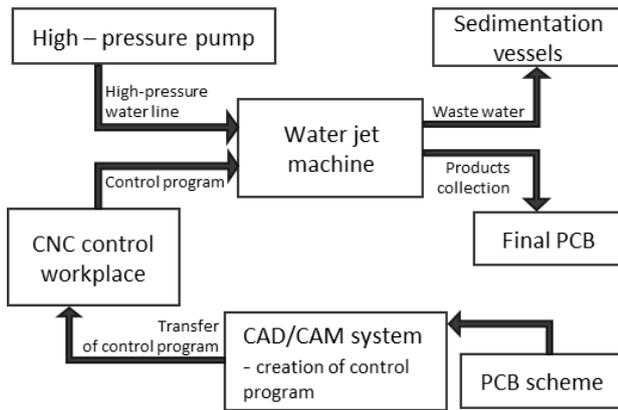
Figure 3. Scheme of PCB production process with WJ technology
