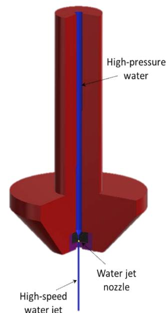
Figure 2. Principle of cutting by clean continuous water jet technology
