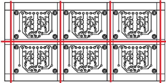
Figure 7. PCB cutting plan
