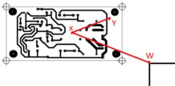
Figure 4. Arrival and departure of the cutting head
