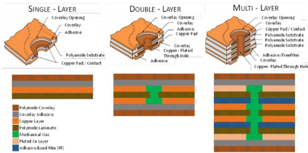
Figure 1. PCB cross-section [8]
