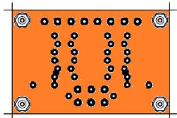
Figure 5. Designed PCB holes
