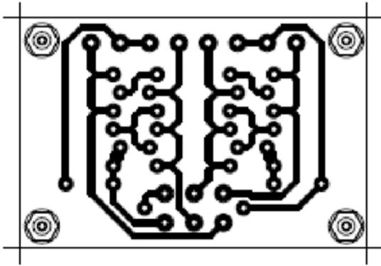
Figure 6. PCB conductive pattern
