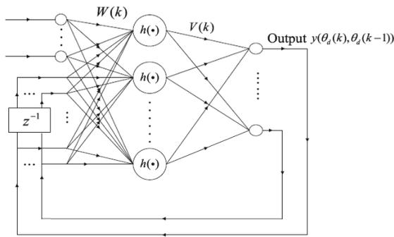
Figure 7. Structure for external feedback RNN
