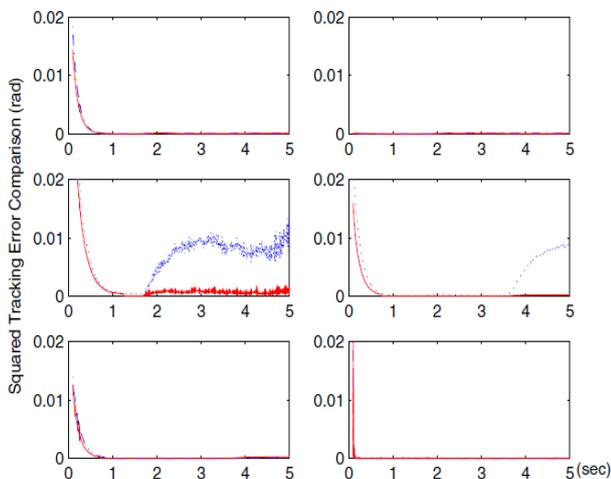
Figure 9. Squared Tracking Error in case of fault occurring (Red/ Straight line with RNN, Blue/ Dashed line without RNN) [11].
