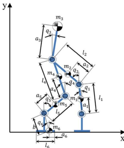
Figure 2. Physical structure of Biped Robot
