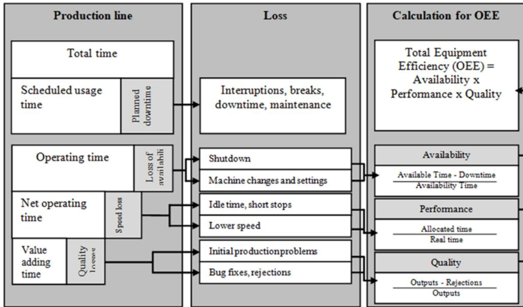
Figure 2. Basic elements and parameters OEE
