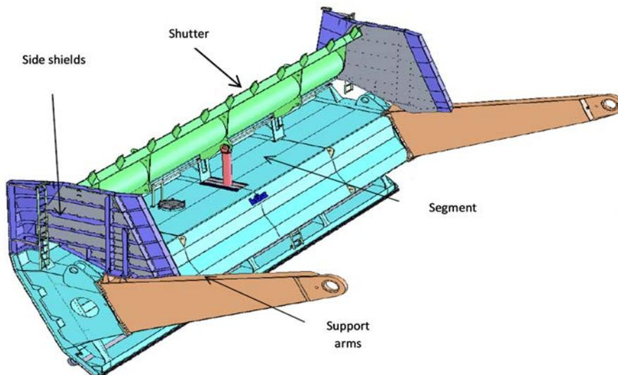
Figure 5. 3D assembly model
