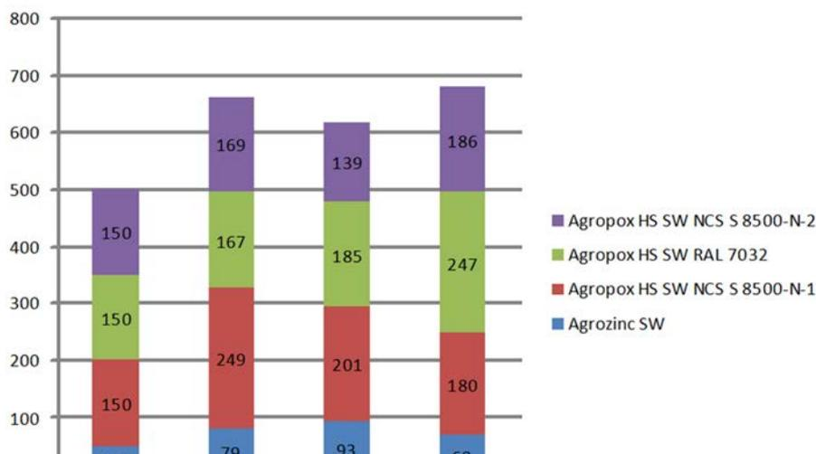
Figure 7. Colour Thickness - Water Side
