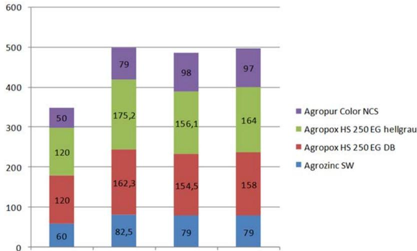
Figure 6. Applied paint thickness on the air side
