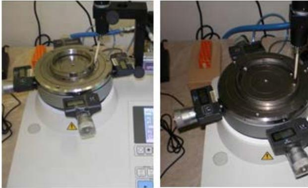
Figure 9. Measurement of the circularity on the raceways of the inner and outer ring
