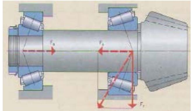
Figure 1. Assembly of the bearing with axial prestress
