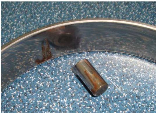
Figure 4. Local surface corrosion on the shell of the rolling element
