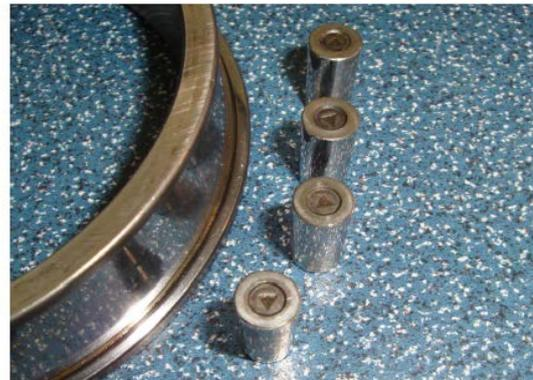
Figure 6. Abrasion on the faces of the rolling elements and on the face of the inner ring
