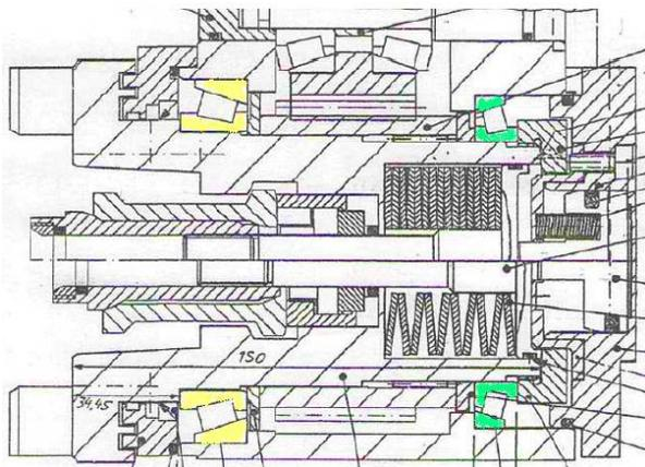
Figure 3. Tapered roller bearings
