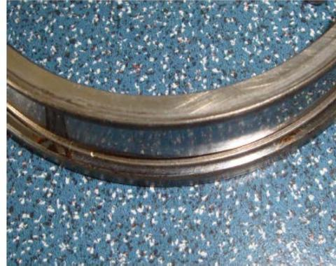
Figure 5. Local surface corrosion on the inner ring
