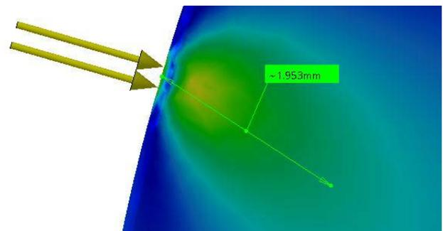
Figure 10. Depth of Hertz pressure ( $F = 2500$  N, full body gear tooth)
