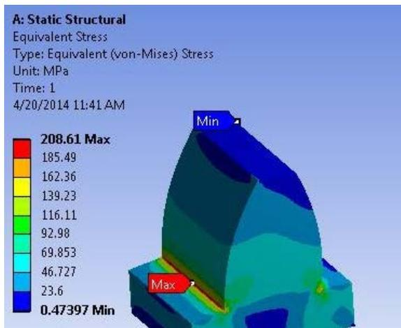
Figure 8. Vonn-Misses stress results in gear root area from [16]
