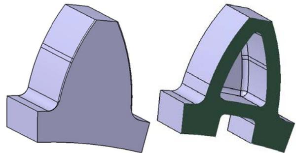
Figure 5. Full body tooth (a), shell body tooth (with a section view) (b).
