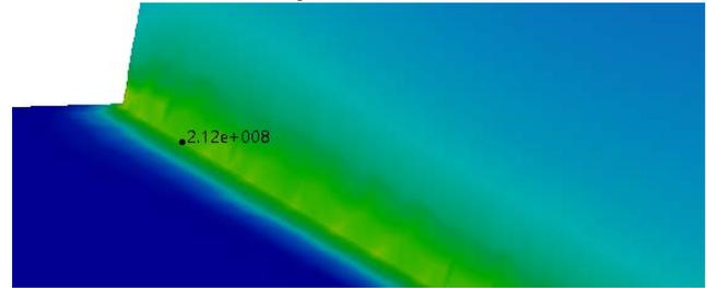
Figure 9. Vonn-Misses stress results in gear root area from this research
