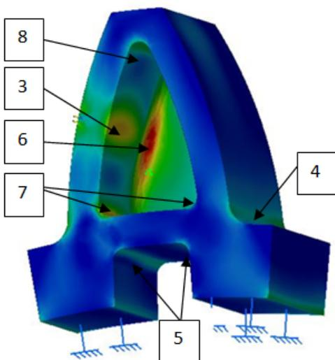
Figure 12. Von-Misses stress of shell body gear tooth. Places of analysis (increased stress).
