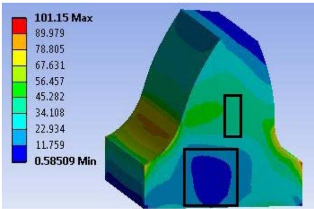
Figure 4. Von-Mises stress in contact region and the tooth root. [16]
