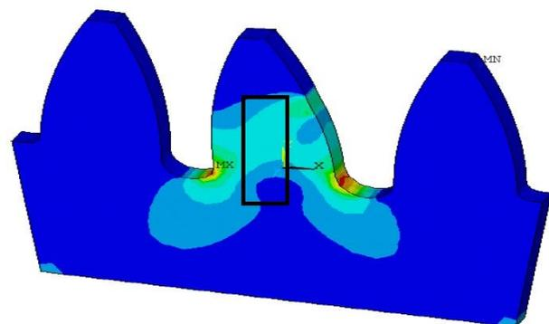
Figure 3. Principal stress in contact region and the tooth root. [15]
