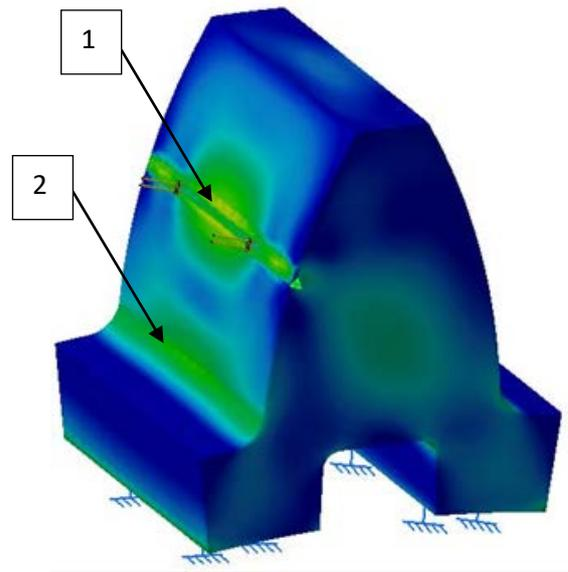
Figure 11. Von-Misses stress of shell body gear tooth. Places of analysis (increased stress).
