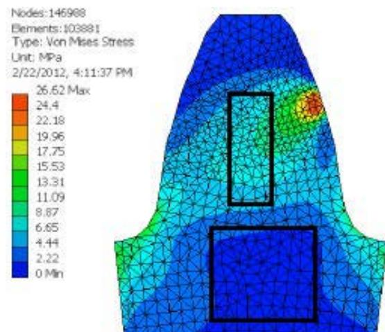
Figure 2. Von-Mises stress in contact region and the tooth root. [13]
