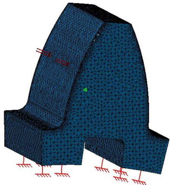
Figure 6. FEM model of gear tooth
