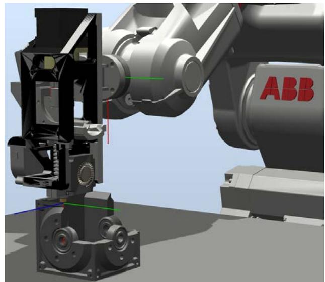
Figure 5. Visualization of 3D printhead with extruder and print object
