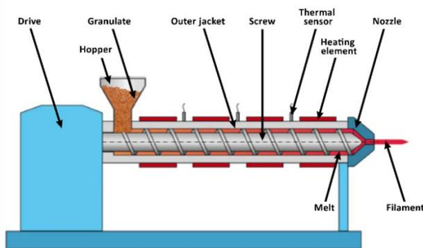
Figure 2. Filament production process from granulate
