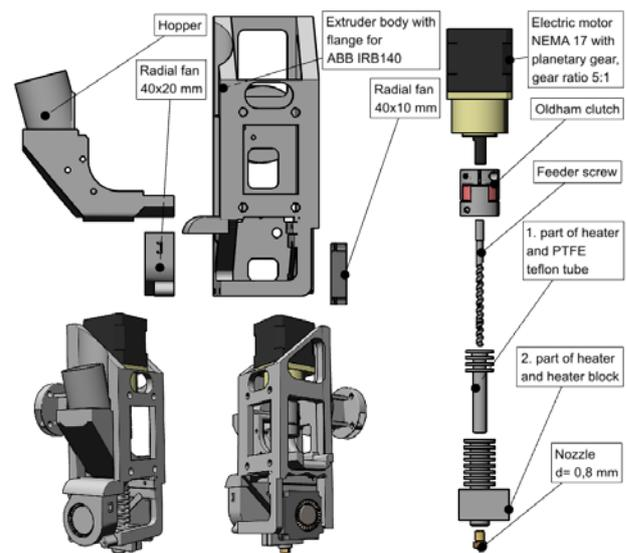
Figure 3. Basic parts of the designed printhead with extruder
