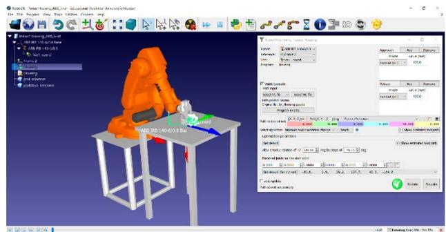
Figure 6. Implementation of simulation and program generation design for 3D printing needs by selected industrial robots in the software RoboDK
