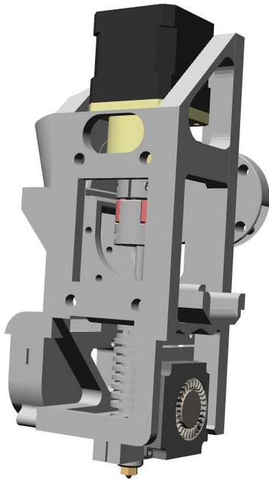
Figure 4. Final design of the proposed printhead with extruder in 3D view
