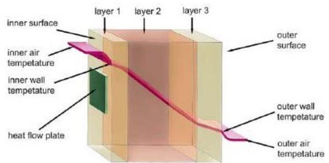
Figure 1. Illustration of the heat flow plate on the wall and parameters – indoor air and wall temperature, outside air and wall temperature.
