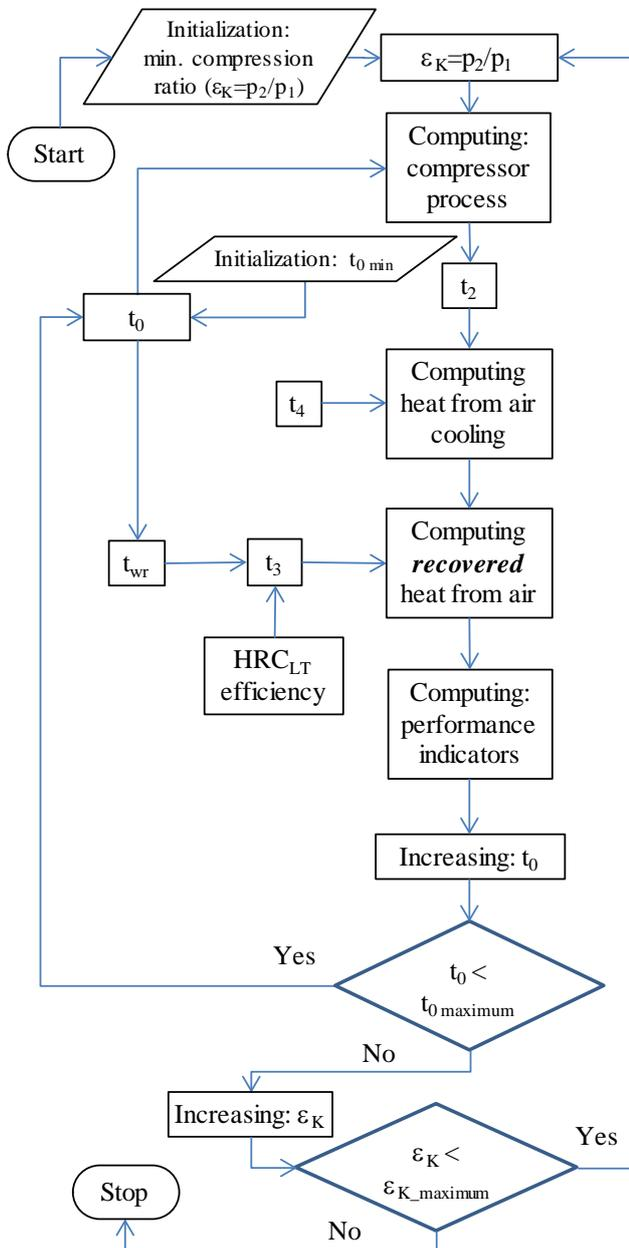
Figure 7. Flow-chart for modelling the compression and aftercooling process and the recovered heat from air
