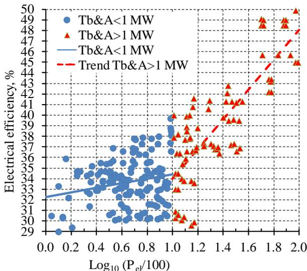
Figure 5. Electrical efficiency vs. RICE power
