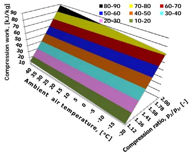
Figure 8. Compression work (kJ/kg) vs. ambient air temperature ( $^\circ\text{C}$ ) and compression ratio (-)
