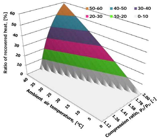
Figure 12. Ratio of recovered heat from air aftercooling process vs. air temperature, and compression ratio
