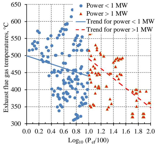
Figure 6. Exhaust flue gas temperatures ( $^\circ\text{C}$ ) vs. RICE power
