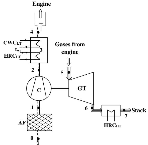
AF – air filter, C – compressor,  $HRC_{LT}$  - heat recovery circuit at low temperature,  $CWC_{LT}$  - cooling water circuit at low temperature, GT – gas turbine,  $HRC_{HT}$  - high temperature flue gases heat recovery circuit
