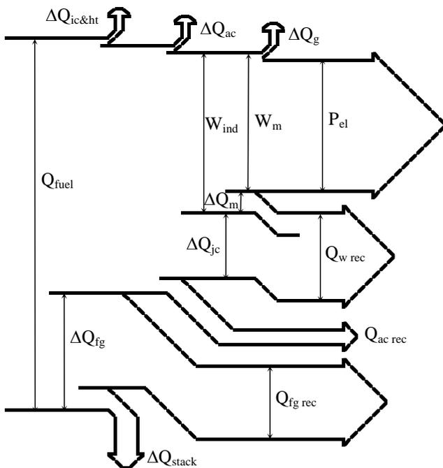
$Q_{ac\ rec}$  – heat flow rate recovered from compressed gas & air cooling,  $\Delta Q_{ac}$  –heat flow rate unrecovered from compressed gas & air cooling.
