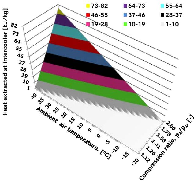
Figure 10. The amount of heat taken over at aftercooler per 1 kg air, versus air temperature, and compression ratio
