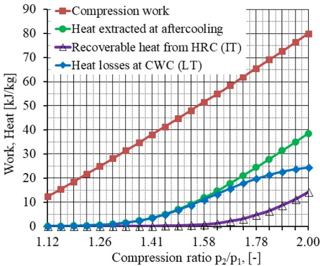
Figure 14. Average annual values of compression work, heat extracted at aftercooling, recoverable heat from HRC<sub>LT</sub>, and heat losses at CWC [kJ/kg]. (HRC cu LT)
