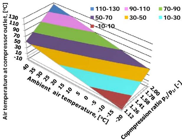
Figure 9. Air temperature at compressor outlet, versus ambient air temperature, and compression ratio
