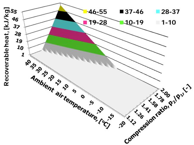
Figure 11. Recoverable heat from air aftercooling process per 1 kg, versus ambient air temperature, and compression ratio
