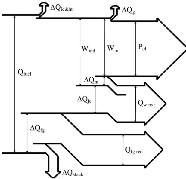
$Q_{fuel}$  – fuel heat flow rate,  $W_{ind}$  – indicated work,  $W_m$  – mechanical work,  $P_{el}$  – power at generator’s clamps,  $Q_{w\ rec}$  – heat flow rate recovered from liquid cooling circuit,  $Q_{fg\ rec}$  – heat flow rate recovered from flue gases,  $\Delta Q_m$  – mechanical losses,  $\Delta Q_{jc}$  – jacket cooling losses,  $\Delta Q_{fg}$  – sensible heat of gases;  $\Delta Q_{stack}$  – stack losses.
