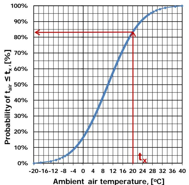
Figure 13. Probabilistic distribution of ambient air temperatures in the average climate conditions of Romania
