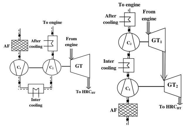
a) 2 stage compression turbocharger with a single turbine and 2 compressors
