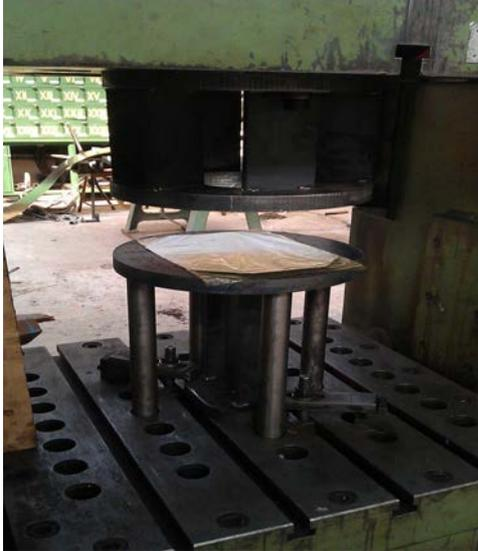
Figure 6. Tensoning tool for deep pulling
