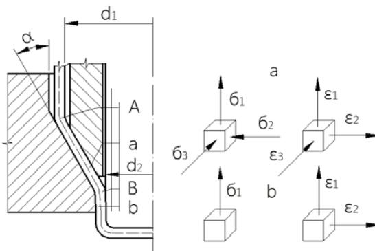
Figure 2. Draw and deformation schemes for drawing cylinders for second and other pulling operations
