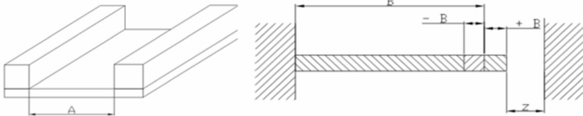
Figure 11. Distance between guide bars
