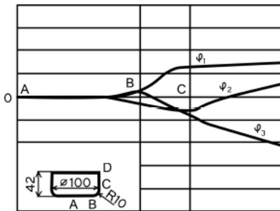
Figure 1. Scheme of the course of logarithmic deformations in drawing cylinders
