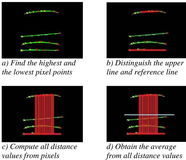
Figure 5. Feature extraction method for a misplaced cap
