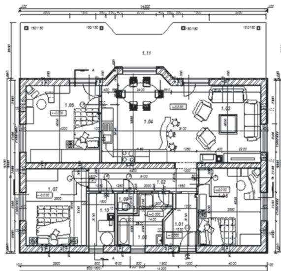
Figure 2. The ground-plan of the single-story family house
