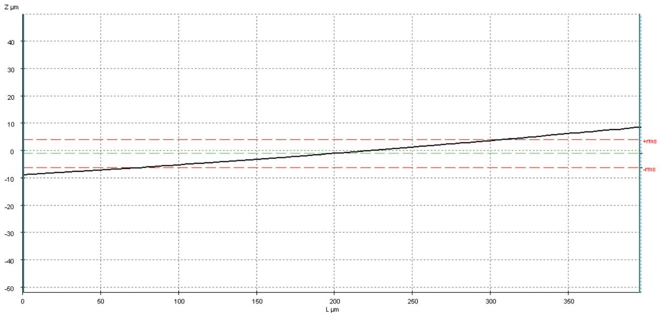
Fig.7. Thickness of TiCN layer measured using 3D confocal microscope
