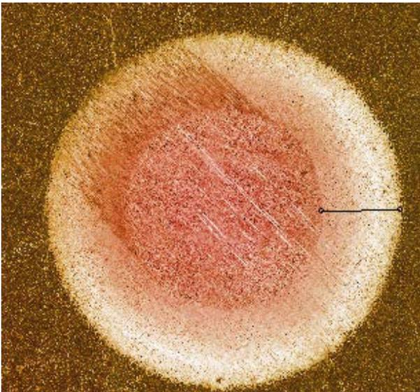
Fig.8 Imprint image of calotest with marked place for TiCN coating thickness measurement
