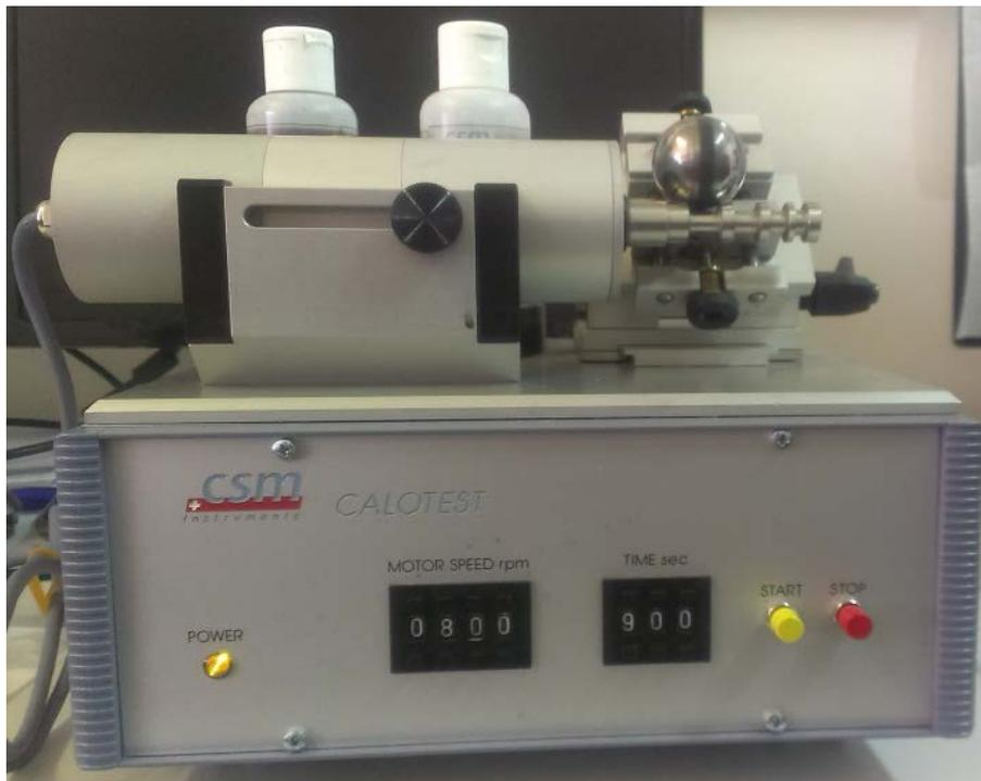
Fig.4 Calotest device form manufacturer CSM
