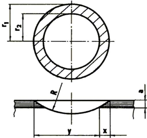
Fig .3 Measured parameters of imprint in deposited layer after calotest [2]
