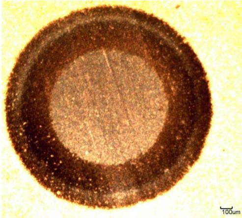
Fig.5 Imprint from calotest on CVD layer
