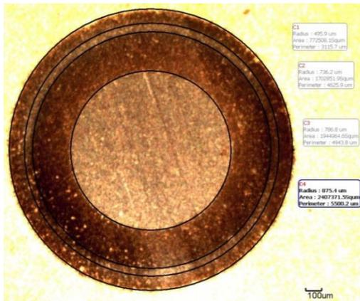
Fig.6 Circle diameters for calculation of layers thickness
