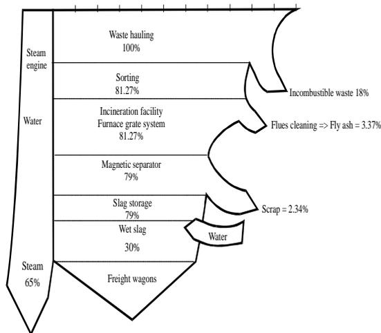
Figure 3. Sankey diagram – a material flow of the waste in waste processing company [27].
