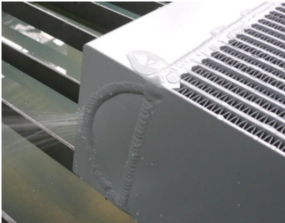
Figure 6. Water leakage from the cooler after the carrying out the Burst test
