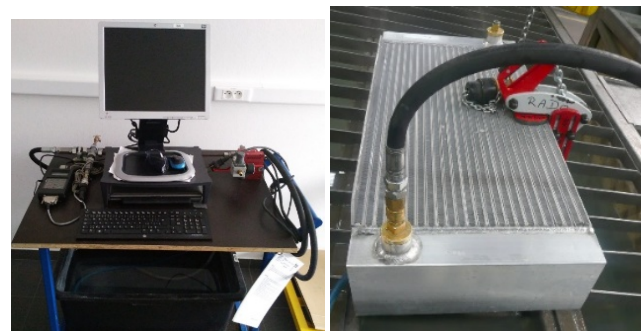
Figure 5. Test station (left) and cooler connection (right)
