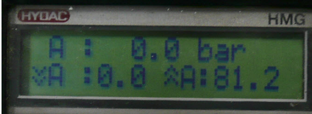
Figure 7. Maximum pressure in the cooler
