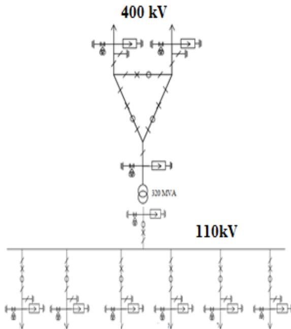
Figure 17. Single-line diagram illustrates the optimal solution of the 400/110kV station, designed from the point of view of the socio-technical systems
