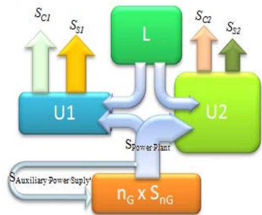
Figure 2. Block diagram (technical perspective) for the evacuation of the electrical energy produced in a power plant with  $n_G$  generators.
