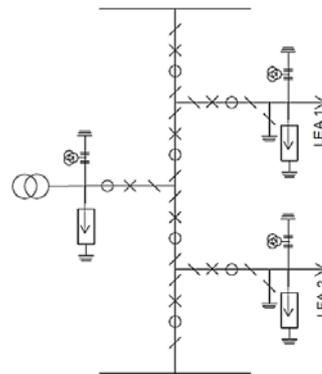
Figure 10. Four breaker for three circuits (1.33 breakers/circuit), AIS, 400kV
