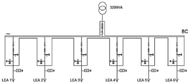
Figure 13. Single bus , GIS, 110 kV
