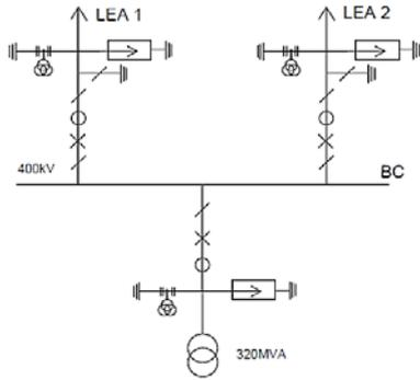
Figure 7. A single bus configuration, AIS, 400kV.
