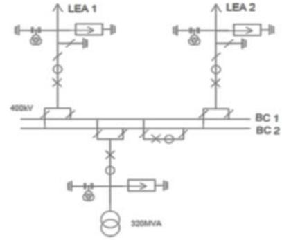
Figure 8. A breaker - double bus configuration, AIS, 400kV.
