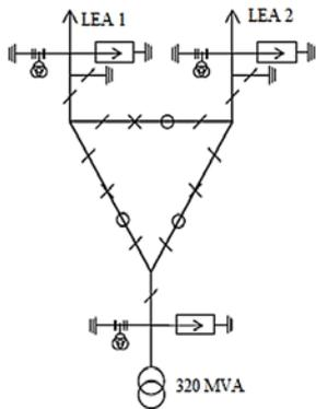
Figure 9. Ring Bus (polygon), AIS, 400kV
