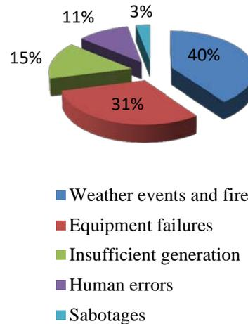
Figure 4. Major Outage Events with Loss of Electric Service, adapted from [23].
