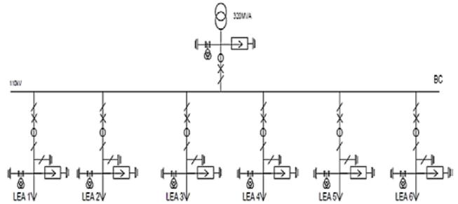
Figure 12. Single bus, AIS, 110 kV
