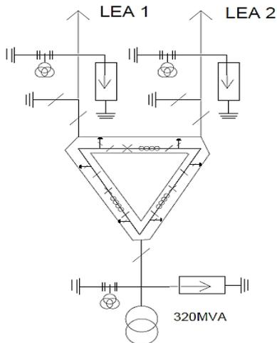
Figure 11. Ring bus (polygon), GIS, 400kV
