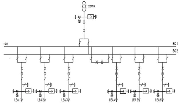
Figure 14. Double bus , AIS, 110 kV
