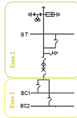
Figure 6. Demarcation example of the two zones of a cell (in switching scheme solutions with  $2BC+BT$ ) for the calculation the penalties for non-delivery of power energy.
