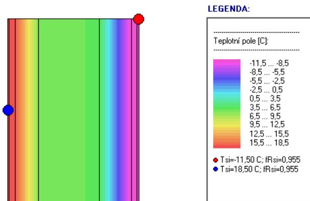
Figure 2. Temperature field Quadlock
