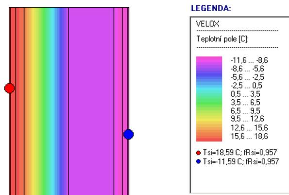
Figure 4. Temperature field Velox WS
