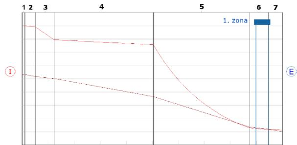
Figure 3. Distribution of water vapor pressures Velox WS
