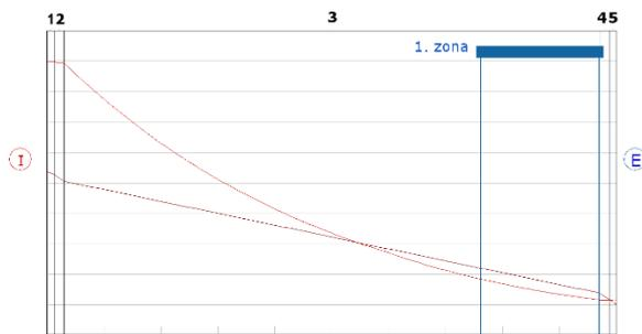
Figure 5. Distribution of water vapor pressures Ytong
