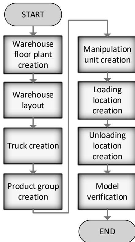
Figure 2. Simulation model creation procedure
