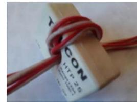
Figure 11. Differential current sensor with twisted yarn pair for primary winding
