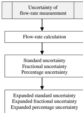
Figure 9. The flow-chart for calculation of flow-rate measurement uncertainty
