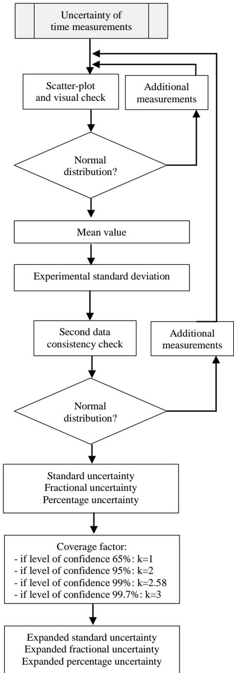
Figure 8. The flow-chart for calculation of time measurements uncertainty
