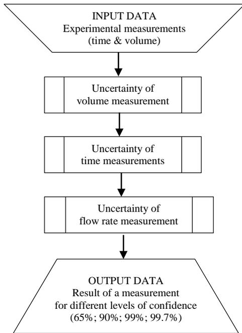
Figure 6. The methodology for calculation of flow-rate uncertainty for repeated measurements
