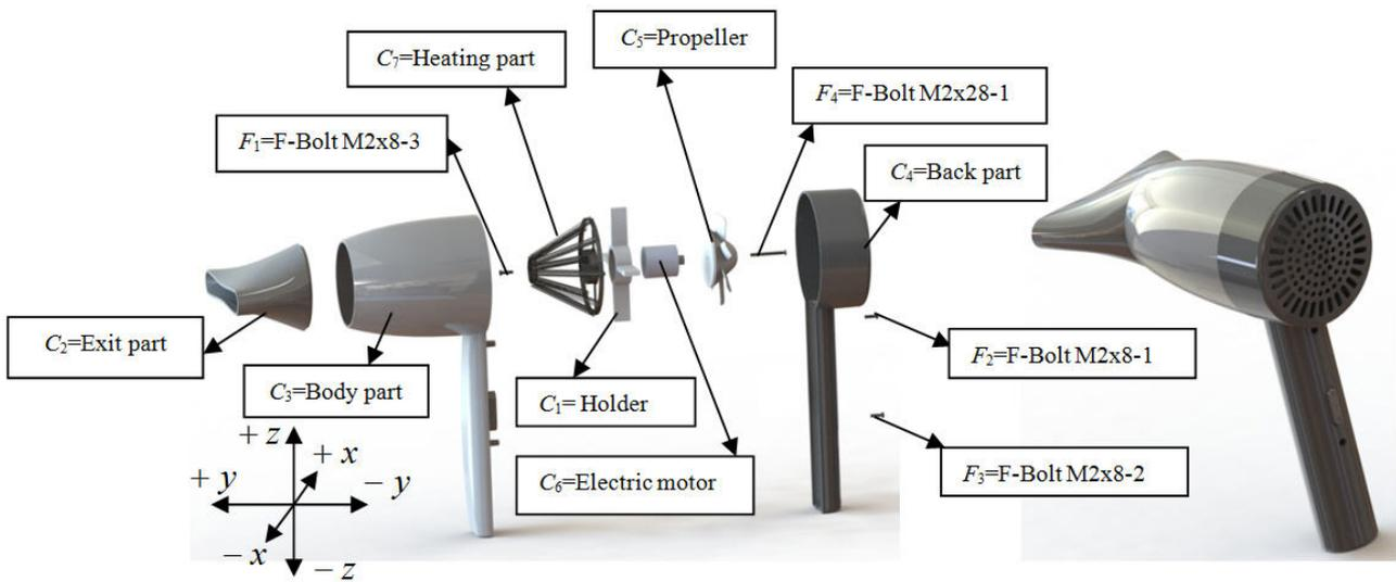
Figure 2. Exploded view and assembly of hair-dryer
