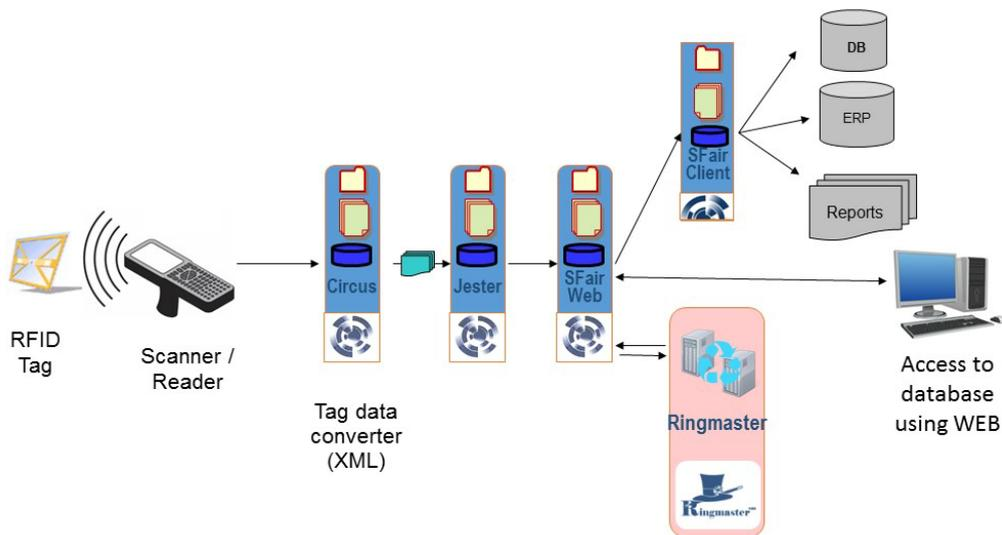
Figure 3. Diagram of the RFID software system architecture
