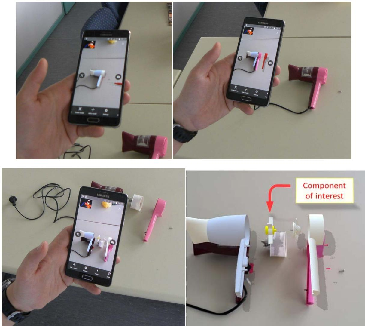
Figure 5. Step-by-step visual guide for nondestructive disassembly operations in Augmented Reality
