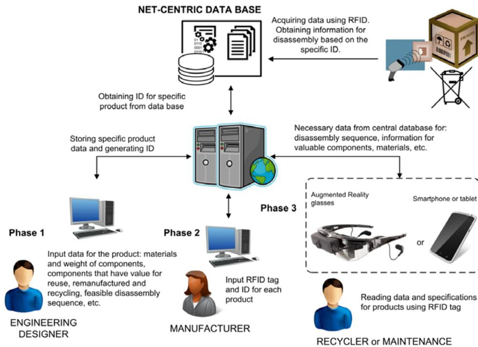
Figure 1. Flowchart of the proposed model for nondestructive disassembly using augmented reality and RFID technology
