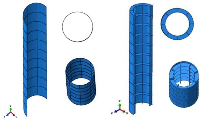
steel shell model is used as a first case (Case I) and the second case (Case II) consists of extra plates which are used for strengthening of thin-walled steel structures.
