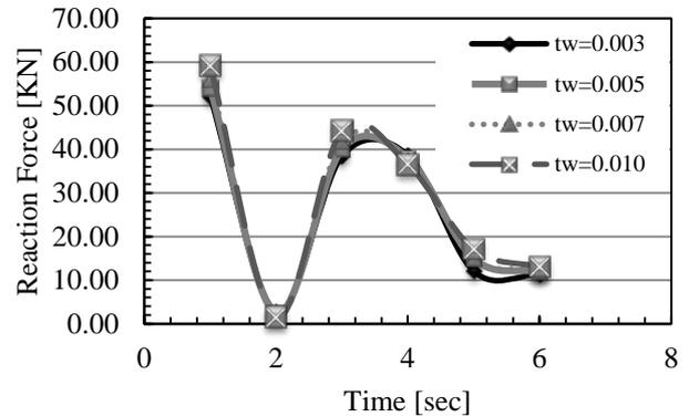
Figure 11. The distribution of reaction force values for Case II
