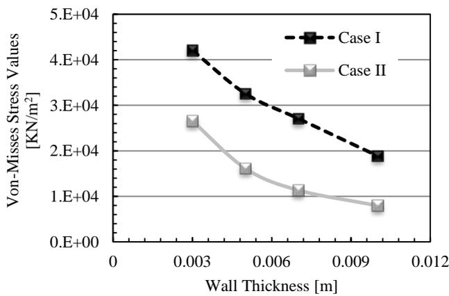
Figure 7. The stress distribution depending on the wall thickness at level -5m when  $t = 3s$
