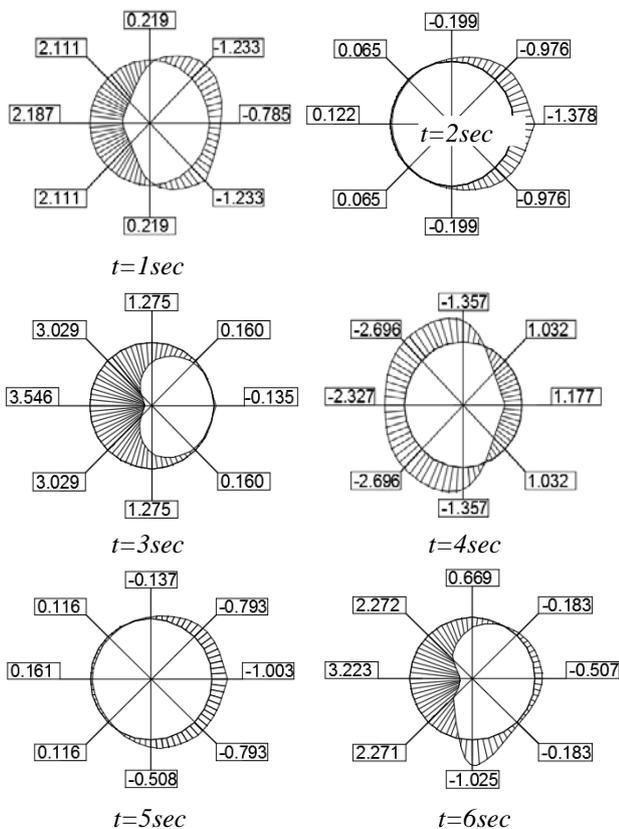
Figure 5. The pressure ( $\text{KN/m}^2$ ) distribution on Cylindrical structure surface at level -5m
