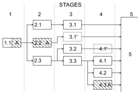
Fig. 1 Diagram of the flow of parts in a machine production enterprise, incl. automated and non-automated stages
