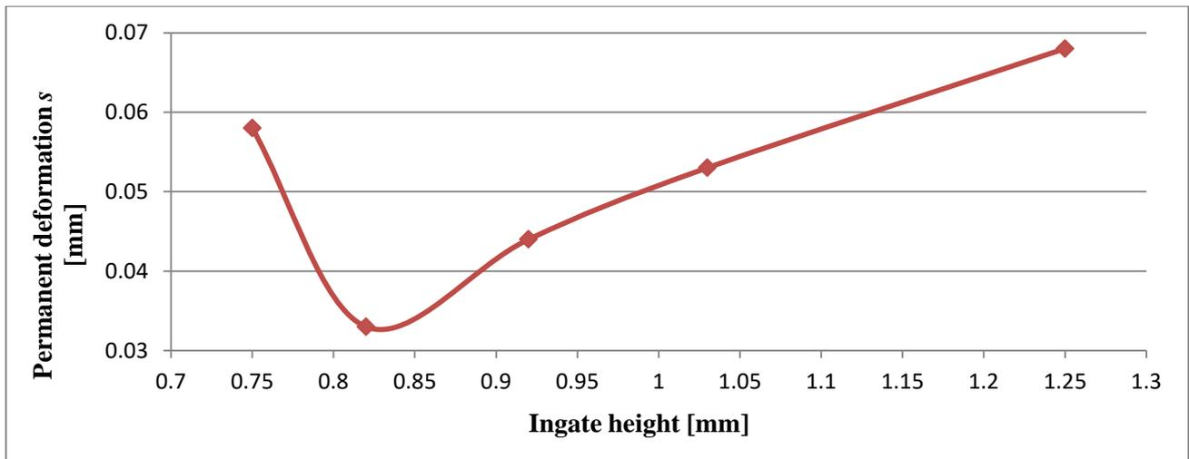
Figure 5. Dependence of permanent deformation  $s$  on the ingate height change
