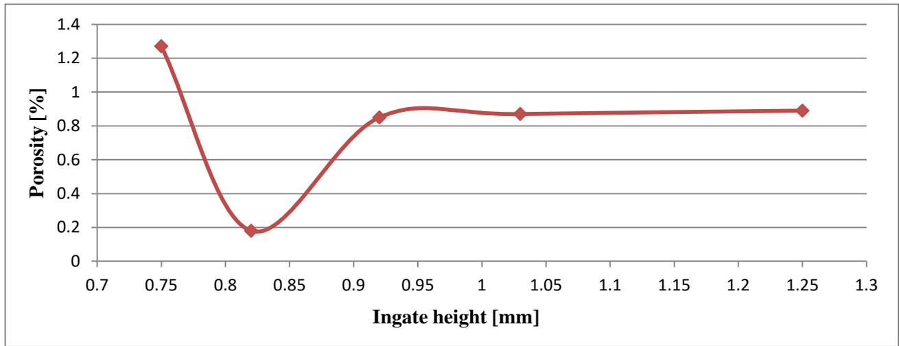
Figure 4. Dependence of porosity  $f$  on the ingate height change
