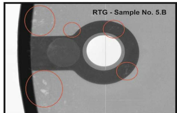
Figure 3. X-ray picture with the highest ration of the cavities
