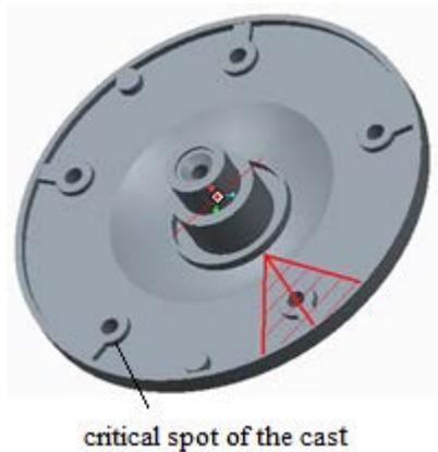
Figure 1. Sampling spot to assess the macrostructure of cast
