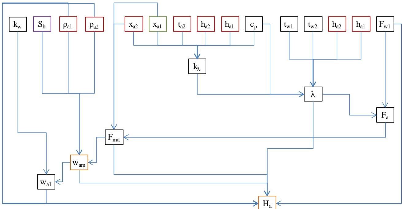
Figure 8. Flow-chart for the height of the rain zone block-module
