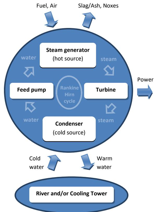
Figure 1. The Rankine-Hirn cycle
