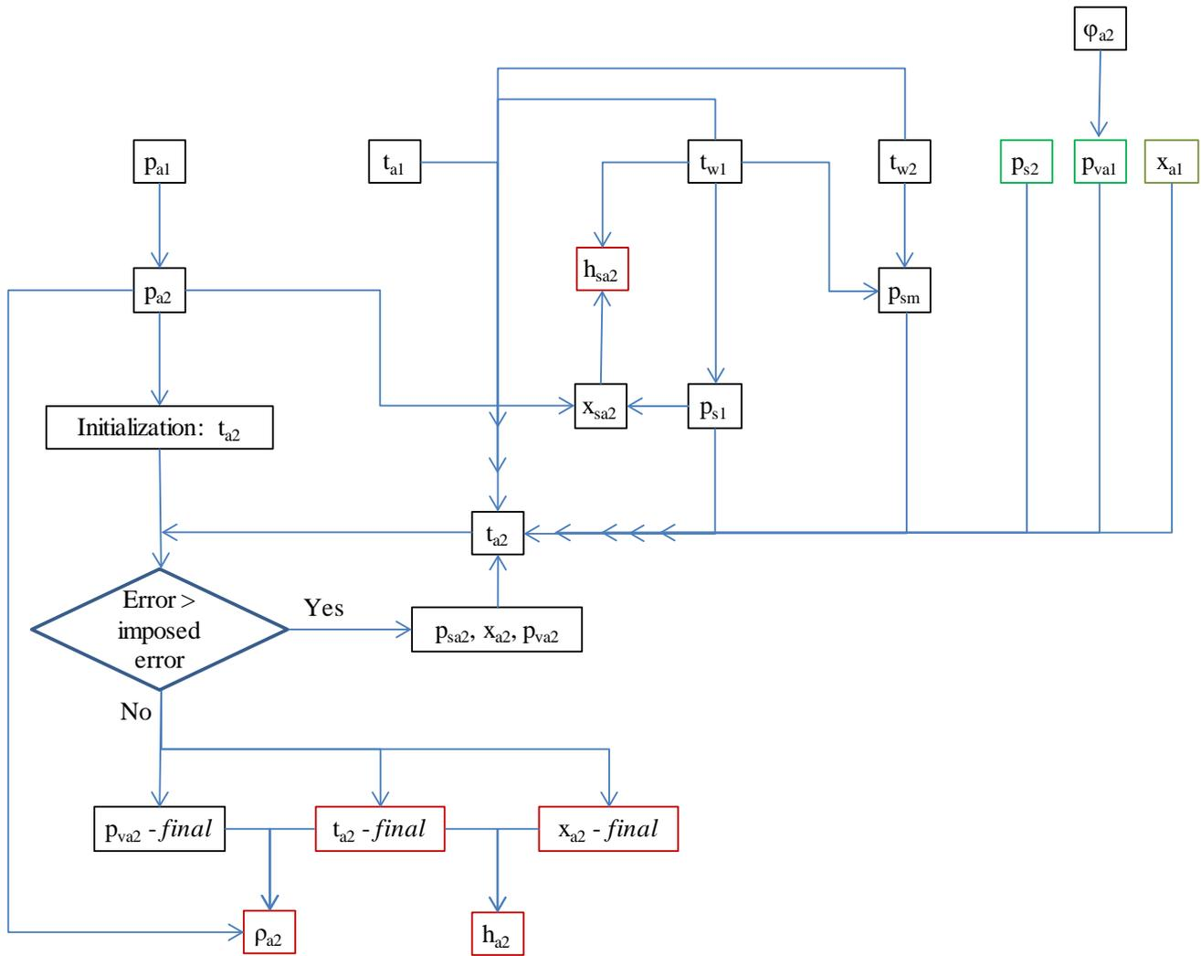
Figure 6. Flow-chart for the outlet air block-module
