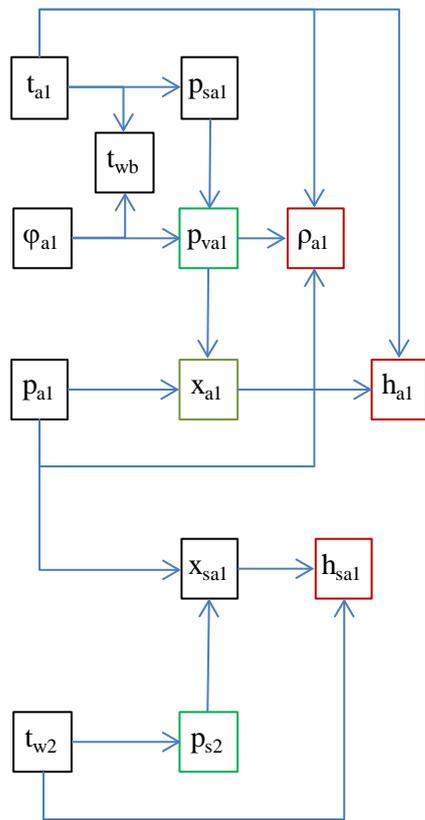
Figure 5. Flow-chart for the inlet air block-module
