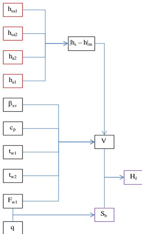
Figure 7. Flow-chart for the height of filling block-module
