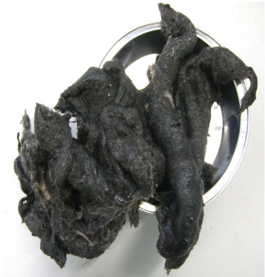
Figure 3. Composite material PVB and fabrics from used tires after homogenization
