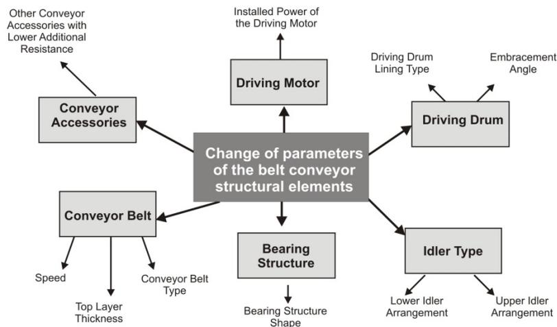
Figure 2. Representation of possible modifications of belt conveyor parameters
