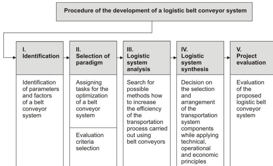
Figure 1. Basic steps within the development of a logistic belt conveyor system
