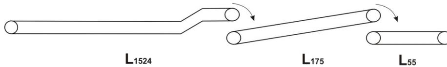
Figure 4. Proposed changes in the route profiles of  $L_{1524}$  and  $L_{175}$  conveyors
