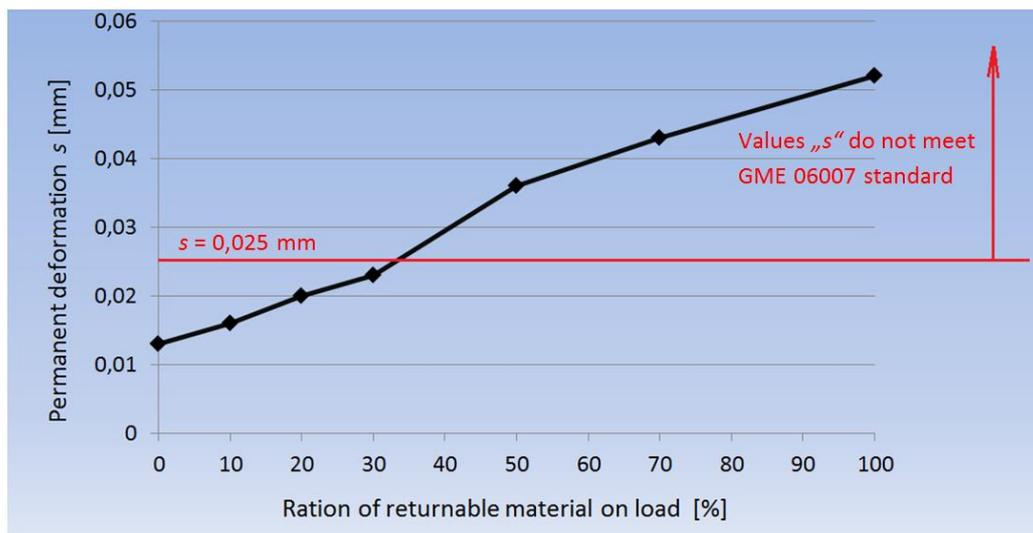
Figure 2. Relation of average values of permanent deformation depending on the percentage ratio of returnable material on load
