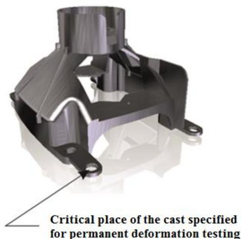
Figure 1. Experimental sample – a pump flange
