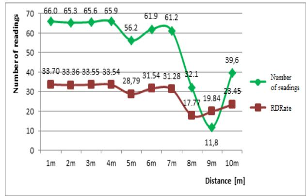
Figure 7. Graph of tag quantitative parameters at 25°C temperature - selected reading distances
