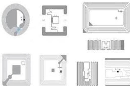
Figure 2. Examples of the most common modification of RFID tags [3]
