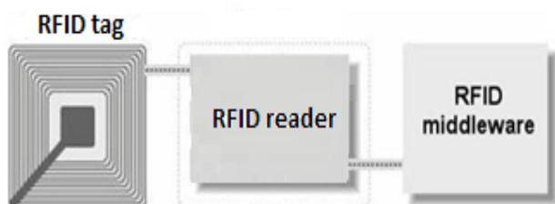
Figure 1. Elements of RFID system [2]
