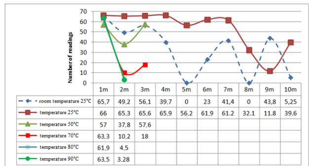
Figure 12. Dependence of Confidex 3000319 tag range from ambient temperature
