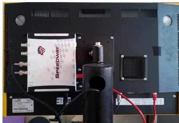
Figure 3. RFID reading device - Impinj Speedway R420
