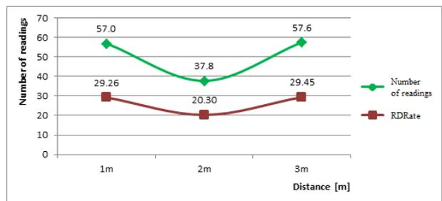
Figure 8. Graph of tag quantitative parameters at 50°C temperature - selected reading distances
