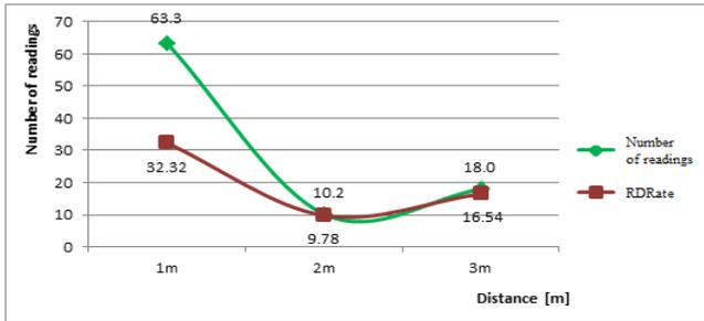
Figure 9. Graph of tag quantitative parameters at 70°C temperature - selected reading distances
