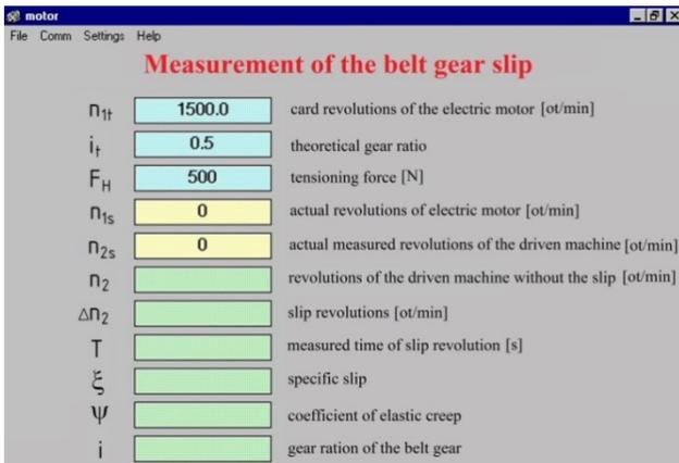
Figure 5. Work area of the software for measurement of the belt gear slip
