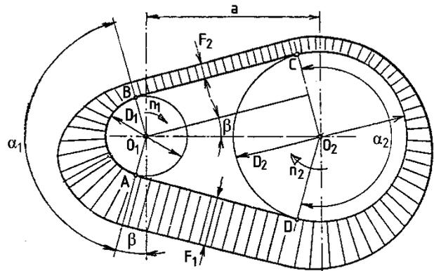
Figure 4. Distribution of forces in case of the belt gear
