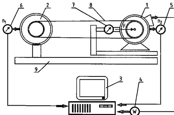
Figure 1. Scheme of measuring device of the belt gear slip: 1 – Electric motor, 2 – Brake, 3 – Computer, 4 – Sensor of output, 5 – Sensor of revolutions  $n_1$ , 6 – Sensor of revolutions  $n_2$ , 7 – Proving ring with deviation meter, 8 – Belt, 9 – Frame
