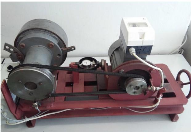
Figure 2. Measuring device of the belt gear slip
