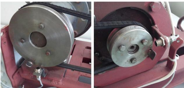
Figure 3. Fixed sensors for measurement of revolutions
