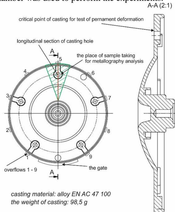
Figure 1. Alternator flange casting
