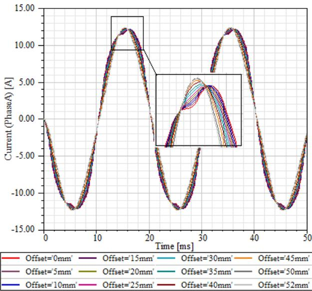
Figure 5. Variation of current in phase A versus time
