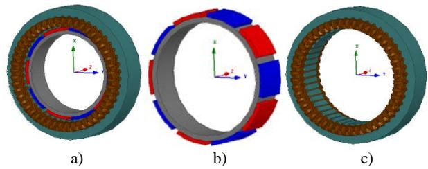
Figure 1.3D models of the generator: (a) Complete view of the generator, (b) Rotor with magnets, (c) Stator with coils.
