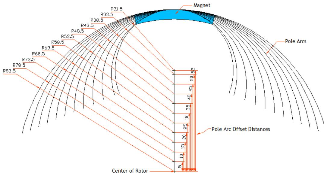
Figure 2.Variation of the parameters of pole arc offset
