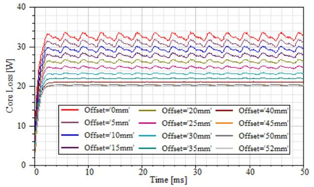
Figure 6. Variation of core loss versus time
