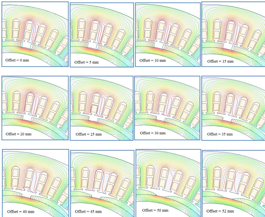
Figure 3.The view of flux lines per offset values and air gaps for 1 kW PMSG
