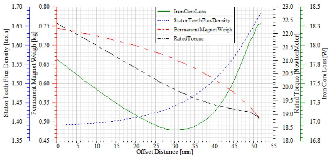
Figure 8. Effect of pole arc offset to rated torque, permanent magnet weight, iron core losses and stator teeth flux density
