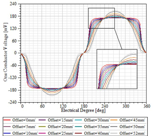
Figure 9. Variation of one conductor voltages and waveforms
