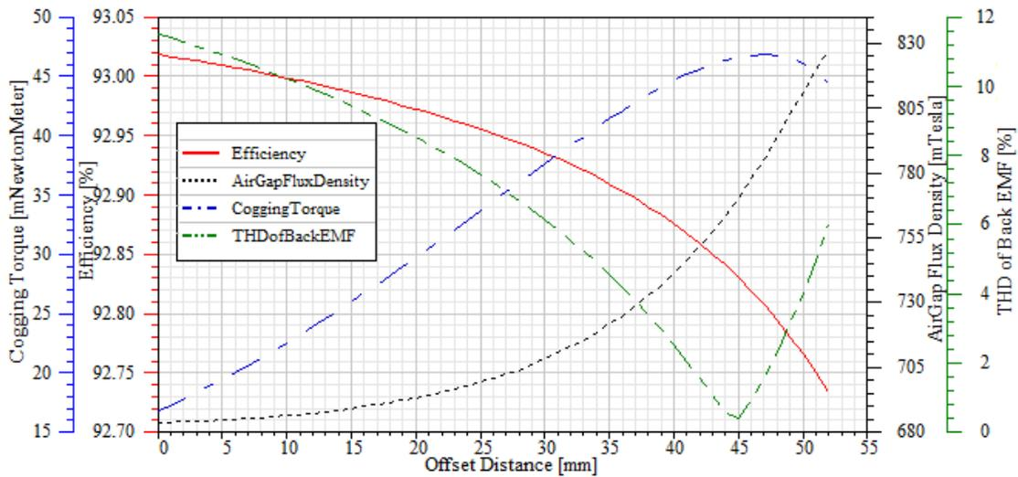
Figure 7. Effect of pole arc offset to efficiency, cogging torque, air gap flux density and THD of back EMF
