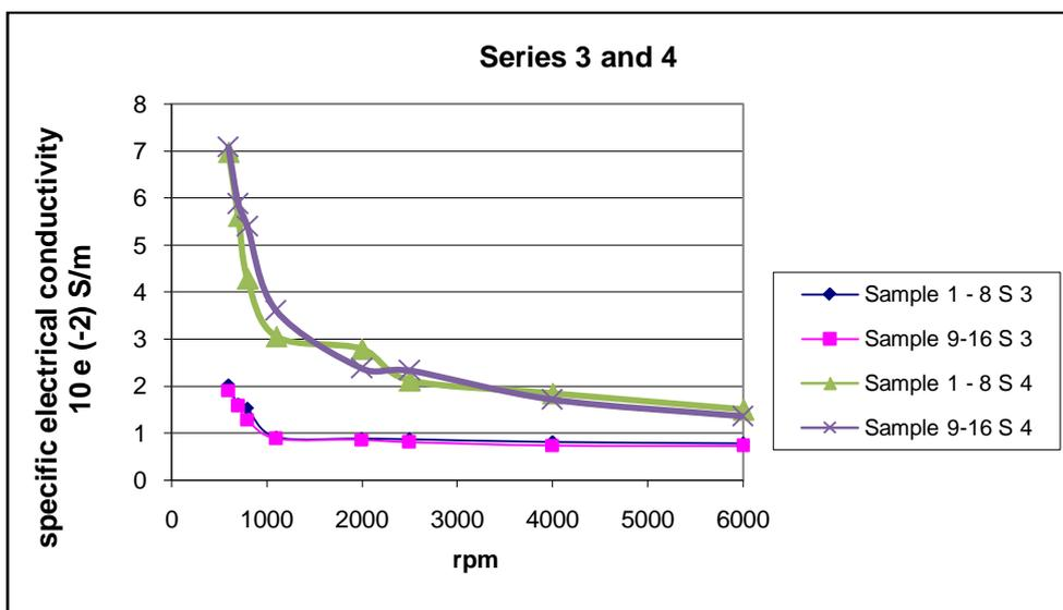
Figure 2. Change in specific electric conductivity depending on the speed of rotation for the thin films PANI-H<sub>2</sub>SO<sub>4</sub> and PANI-HCl obtained at 0°C.
