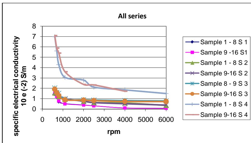
Figure 3. Change in specific electric conductivity depending on the speed of rotation for the thin films PANI-H<sub>2</sub>SO<sub>4</sub> and PANI-HCl for all series.
