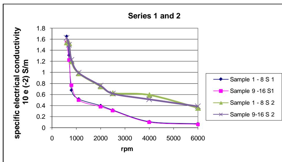
Figure 1. Change in specific electric conductivity depending on the speed of rotation for the thin films PANI-H<sub>2</sub>SO<sub>4</sub> and PANI-HCl obtained at 20°C.
