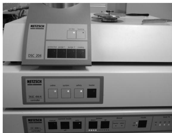
Figure 2. The Equipment DSC 204 NETZSCH [6].
