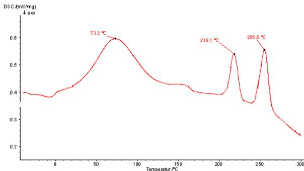
Figure 3. Differential scanning calorimetry of 1<sup>st</sup> heating
