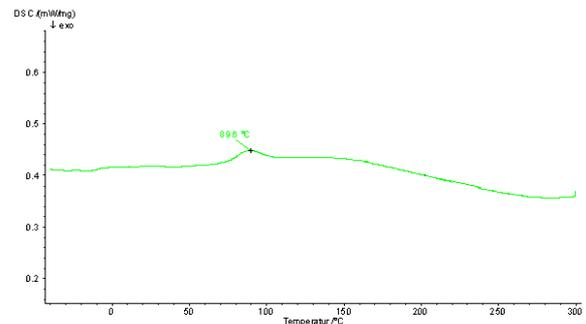
Figure 5. Differential scanning calorimetry of rubber particle
