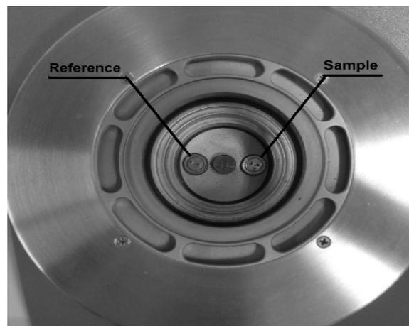
Figure 1. The sample stored in the equipment DSC 204 NETZSCH[6]
