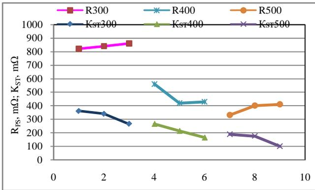
Figure 7. Stability coefficient ( $K_{ST}$ ) and resistance in the output circuit of the plasmatron ( $R_{PS}$ ) by regimes R1 – R9 by  $Q_{MP}=800\text{gr/h}$ .
