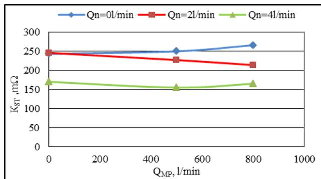
Figure 8. Stability coefficient ( $K_{ST}$ ) as a function of the debit of the metal powder ( $Q_{MP}$ )
