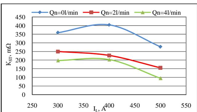
Figure 9. Stability coefficient ( $K_{ST}$ ) as a function of the working current ( $I_L$ )
