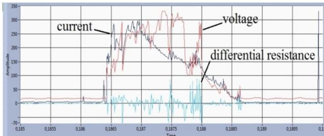
Figure 3. Voltage ( $U_{AK}$ , V) current ( $I_L$ , A) and differential resistance ( $R_D$ ,  $\Omega$ ) in time domain .
