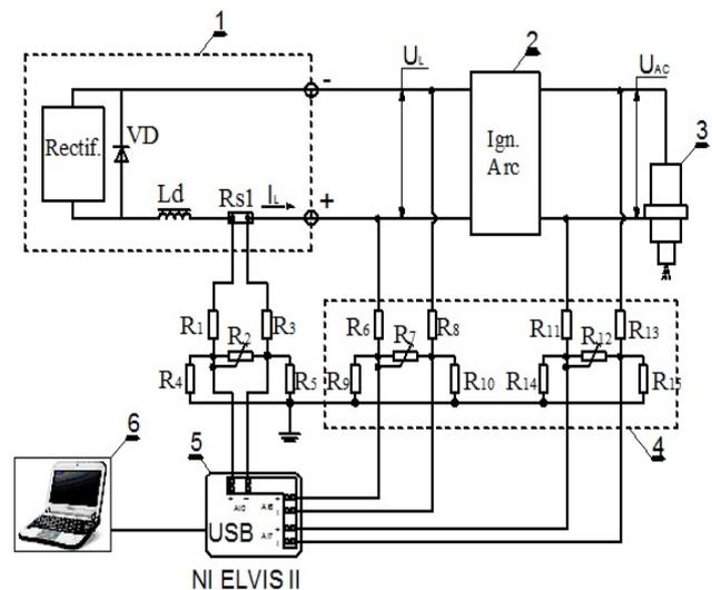
Figure 2. Wiring diagram of the DAQ system and used measuring shunt and voltage dividers for transformation of the signals
