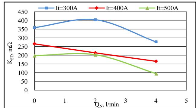
Figure 10. Stability coefficient ( $K_{ST}$ ) as a function of the debit of the additional plasma gas – nitrogen ( $Q_N$ )
