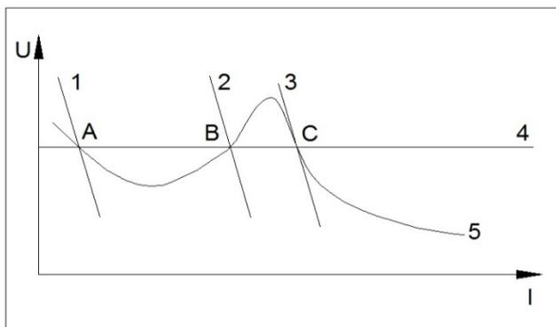
Figure 1. Current-voltage characteristic of the electric arc discharge (5), voltage source(4) and current source (1, 2, 3).
