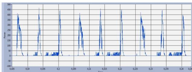
Figure 5. Time domain graphic of the power ( $P_{out}$ , kW), consumed of the plasmatron
