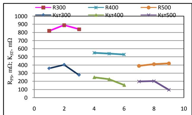
Figure 6. Stability coefficient ( $K_{ST}$ ) and resistance in the output circuit of the plasmatron ( $R_{PS}$ ) by regimes R1 - R9 by  $Q_{MP}=400\text{gr/h}$ .
