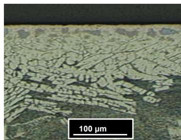
Figure 5. Microstructure of Ti-3Al-2.5V after plasma gas nitriding with 25kW with indirect plasma torch for 3 min - B4.
