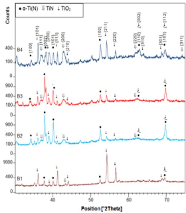
Figure 3. X-ray diffraction patterns for samples B1, B2, B3 and B4 after plasma gas nitriding with indirect plasma torch
