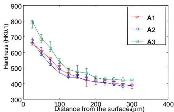
Figure 6. Microhardness profiles of Ti-3Al-2.5V alloy after plasma gas nitriding with 25kW with indirect plasma torch for 3 min for samples A1, A2 and A3.
