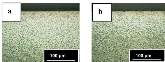
Figure 4. Microstructure of Ti-3Al-2.5V alloy. after plasma gas nitriding with indirect plasma torch (a) B1; (b) B3 - Table 2.
