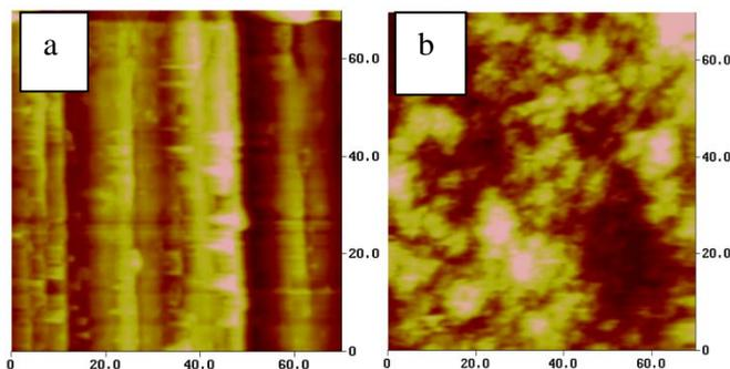
Figure 1. Surface morphology of the samples from the first set before (a) and after (b) plasma gas nitriding with indirect plasma torch at 18kW for 3 min.
