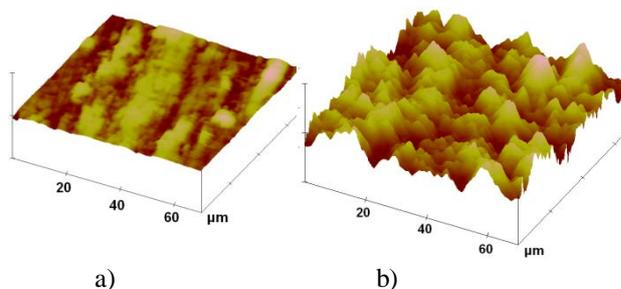
Figure 2. 3D images of the surface morphology of the samples from the second set before (a) and after (b) plasma gas nitriding at 25kW with indirect plasma torch for 3 min.
