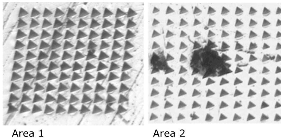
Figure 3. The area of evaluative nano-indentation on the sample's surface
