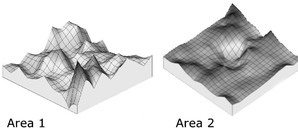
Figure 4. The distribution of hardness on the surface of the investigated areas
