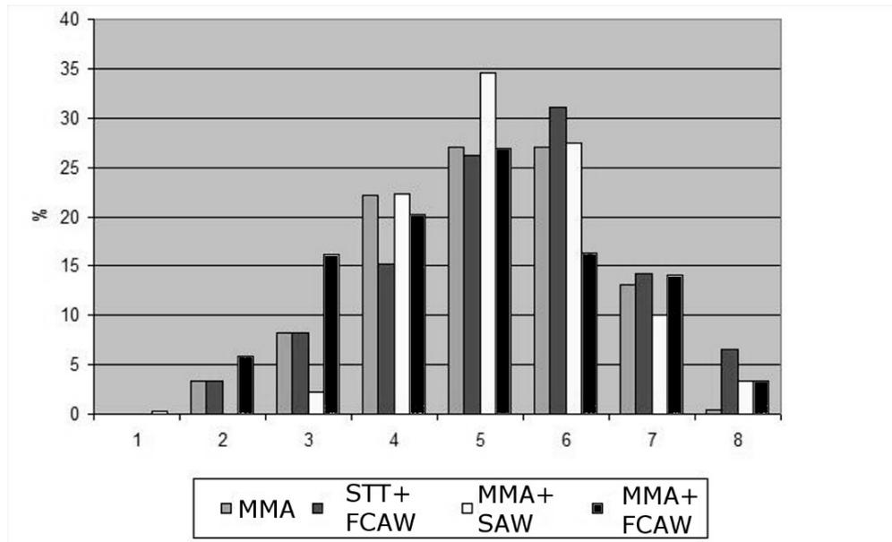
Figure. 1. The concentration of non-metallic inclusions from different size groups in welding joints produced by different ways of welding
