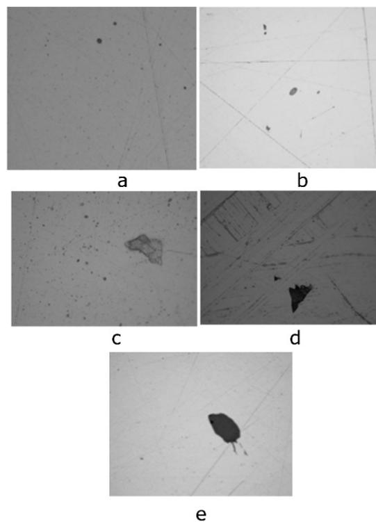
Figure. 2. Non-metallic inclusions investigated by an optical microscope: a – 1-2 size group (x500), b – 3-4 size group (x500), c, d – 5-6 size group (x1000), e – 7-8 size group (x100)
