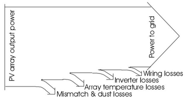
Figure 8. Losses in solar system
