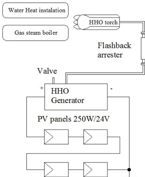
Figure 2. Diagram of the brown gas generator sourced directly from photovoltaic panels
