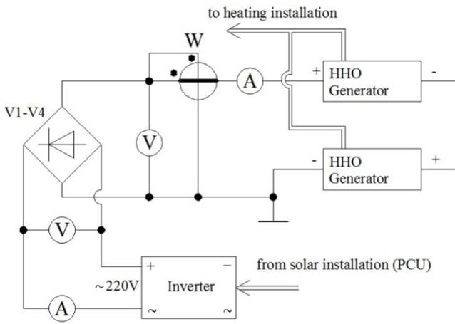
Figure 7. Measurement diagram in BGG electrical feeding with inverter
