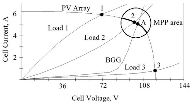
Figure 5. Cross-section between PV characteristic and different type of loads. MPP area.
