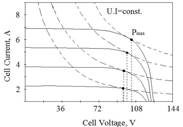
Figure 3. I-V characteristic of the PV panel array
