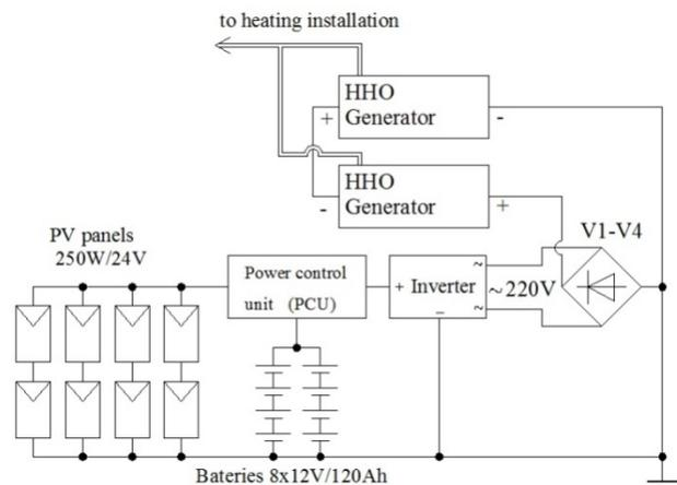
Figure6. Diagram of the brown gas generator sourced with solar system.
