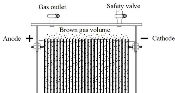
Figure 1. Brown gas generator with serial cells (316L type)
