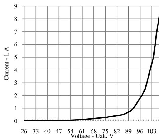
Figure 4. I-V characteristic of the BGG with 53 cells
