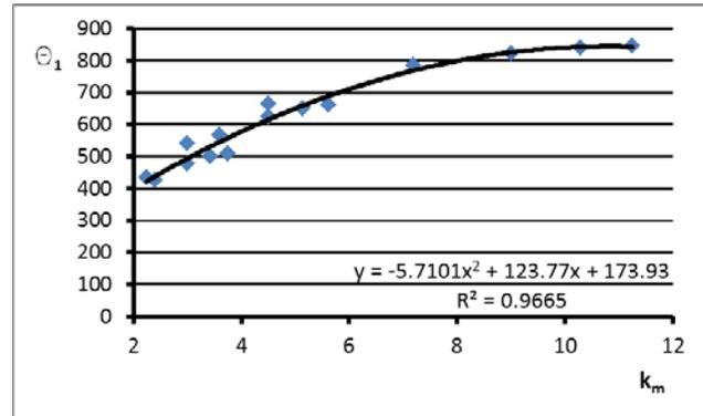
Fig.1 Interpolation relationship between  $k_m$  and  $\theta_1$  for  $t = 60$  minutes and nominal curve ISO 834
