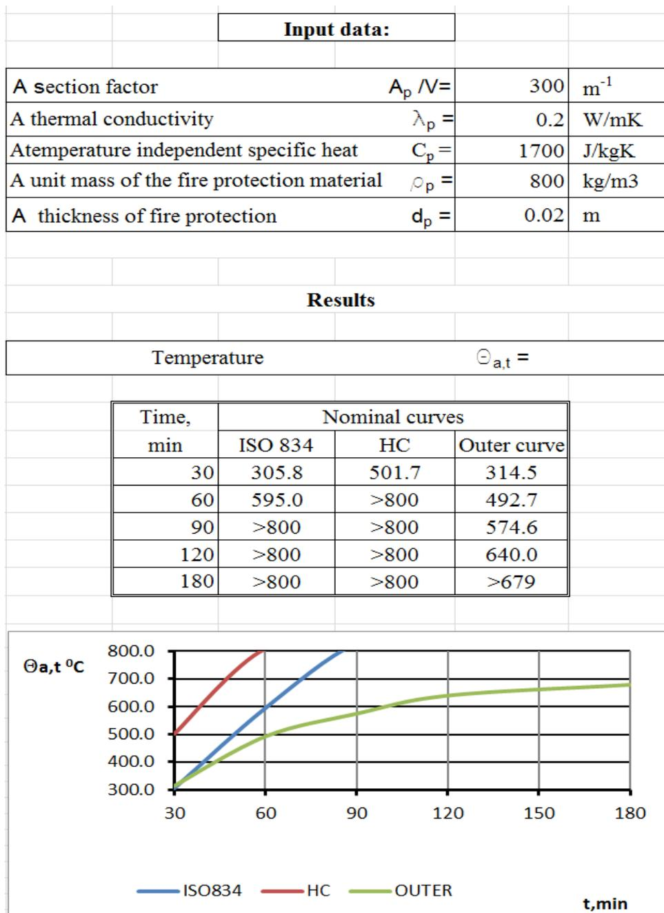
Table 2. Worksheet for the calculation of the temperature of the steel element.
