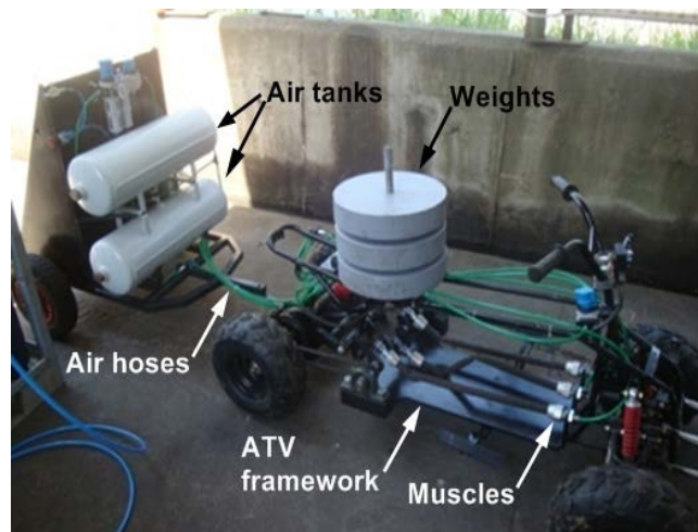
Figure 8. The used weights and preparation of mechanism for test experiments
