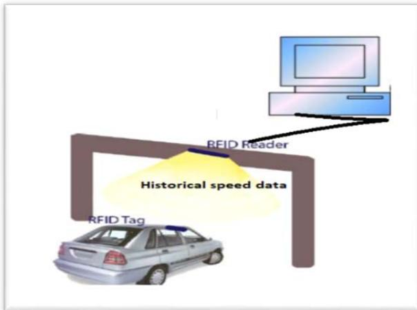
Figure 1. RFID based system for vehicle speed control
