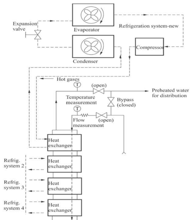
Figure 3. Proposal of solution for installation of heat exchanger for heat recovery from cooling chambers in the production space [18]
